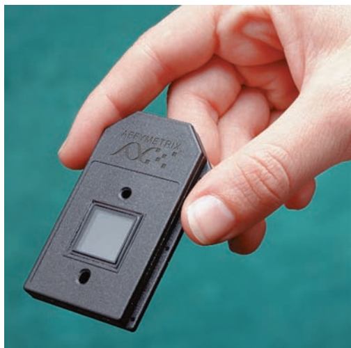
Figure 7-41 A DNA microarray assembly. This so-called GeneChip protects its enclosed DNA microarray and provides a convenient hybridization chamber. To interrogate it requires a specialized fluorescence measurement device. [Courtesy of Affymetrix, Inc., Santa Clara, California.]
