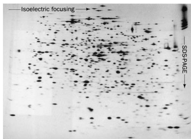
Figure 6-27 Two-dimensional (2D) gel electrophoresis. This autoradiogram shows the separation of E. coli proteins by 2D gel electrophoresis (isoelectric focusing horizontally and SDS-PAGE vertically). A 10- \mu\text{g} sample of proteins from E. coli that had been labeled with ^{14}\text{C} -amino acids was subjected to isoelectric focusing in a 2.5 \times 130 -mm tube of a urea-containing polyacrylamide gel. The gel was then extruded from its tube, placed in contact with one edge of an SDS-polyacrylamide slab gel, and subjected to electrophoresis. Over 1000 spots were counted on the original autoradiogram, which resulted from an 825-h exposure. [Courtesy of Patrick O'Farrell, University of California at San Francisco.]
