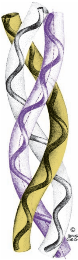
Figure 8-28 The triple helix of collagen. This diagram indicates how the left-handed polypeptide helices are twisted together to form a right-handed superhelical structure. Ropes and cables are similarly constructed from hierarchies of fiber bundles that are alternately twisted in opposite directions. An individual collagen polypeptide helix has 3.3 residues per turn and a pitch of 10.0 Å (in contrast to polyproline II's 3.0 residues per turn and pitch of 9.4 Å; Fig. 8-15). The collagen triple helix has 10 Gly-X-Y units per turn and a pitch of 86.1 Å. [Illustration, Irving Geis. Image from the Irving Geis Collection, Howard Hughes Medical Institute. Reprinted with permission.]
